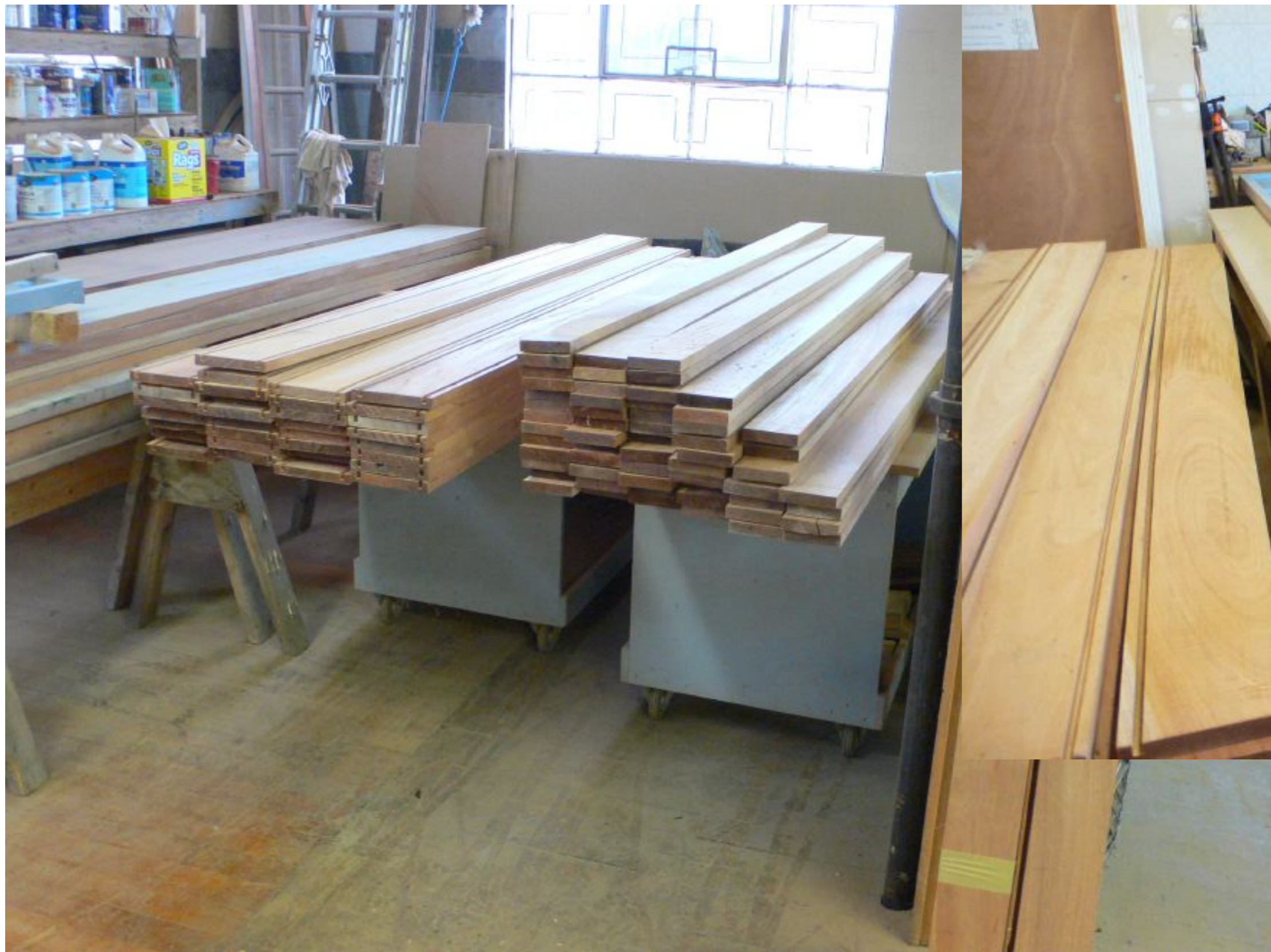
Corner trim boards milling in process (Milled to left), Closeup in right photo
